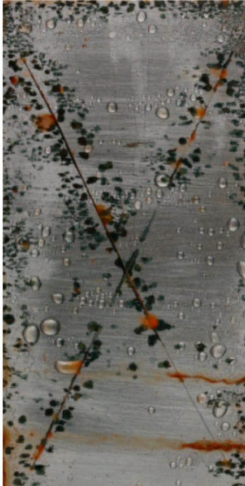
Polyurethane coating protected by AMI Series 1 after 120 hours of salt fog testing (ASTM B117)
